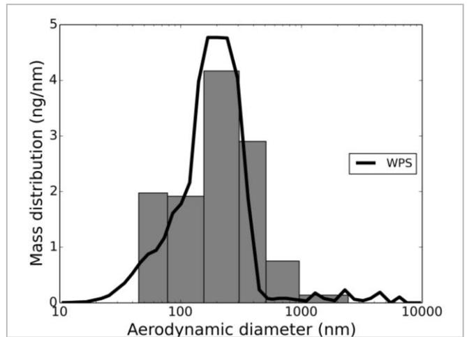
Measurement of ambient aerosol: comparison with Wide-range Particle Spectrometer (1000XP WPS).
