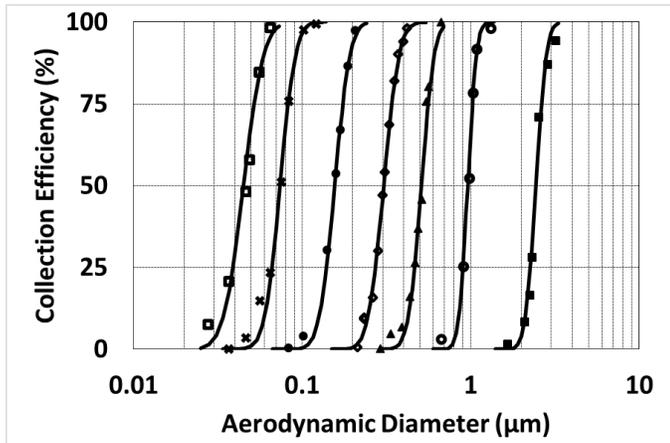
Stage collection efficiency curves measured experimentally with monodisperse aerosols.
