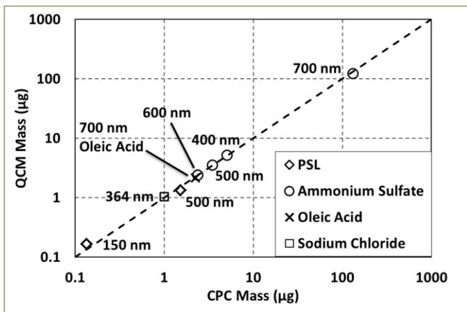
Measurements of laboratory-generated aerosol on a single QCM stage: mass comparison with CPC.
