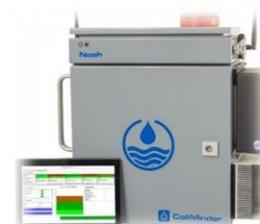
Measurements of the overall activity of the ColiMinder instrument are very sensitive and it cannot happen that the instrument shows a negative result, while laboratory analysis of HPC would be positive. In addition to microbiological activity, the device also measures the transparency of water. Transparency is a suitable additional indicator for monitoring the production process.
