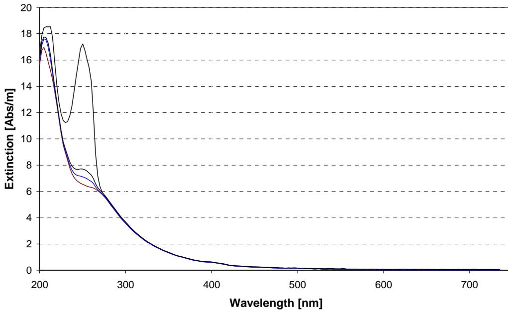
**Figure 3.4:** Absorption spectra of drinking water contaminated with benzene. From top to bottom benzene concentrations are 1 mg/L, 0.1 mg/L, 0.05 mg/L and 0 mg/L.
