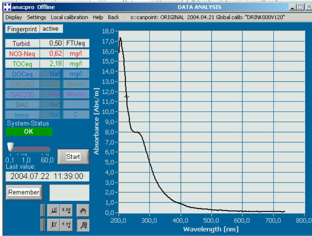
Figure 2.6: Display for viewing results of measured fingerprint spectra.
