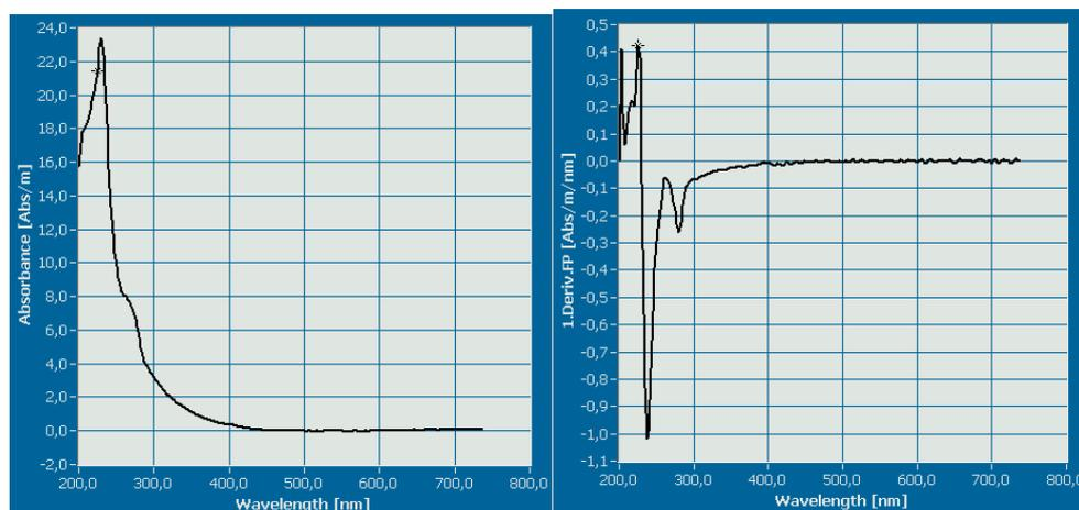
**Figure 3.9:** Fingerprint spectrum of 5 mg/L benzoic acid in drinking water (left) and the 1<sup>st</sup> derivative spectrum (right).
