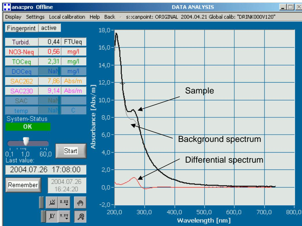
Figure 3.8: Differential spectroscopy.
