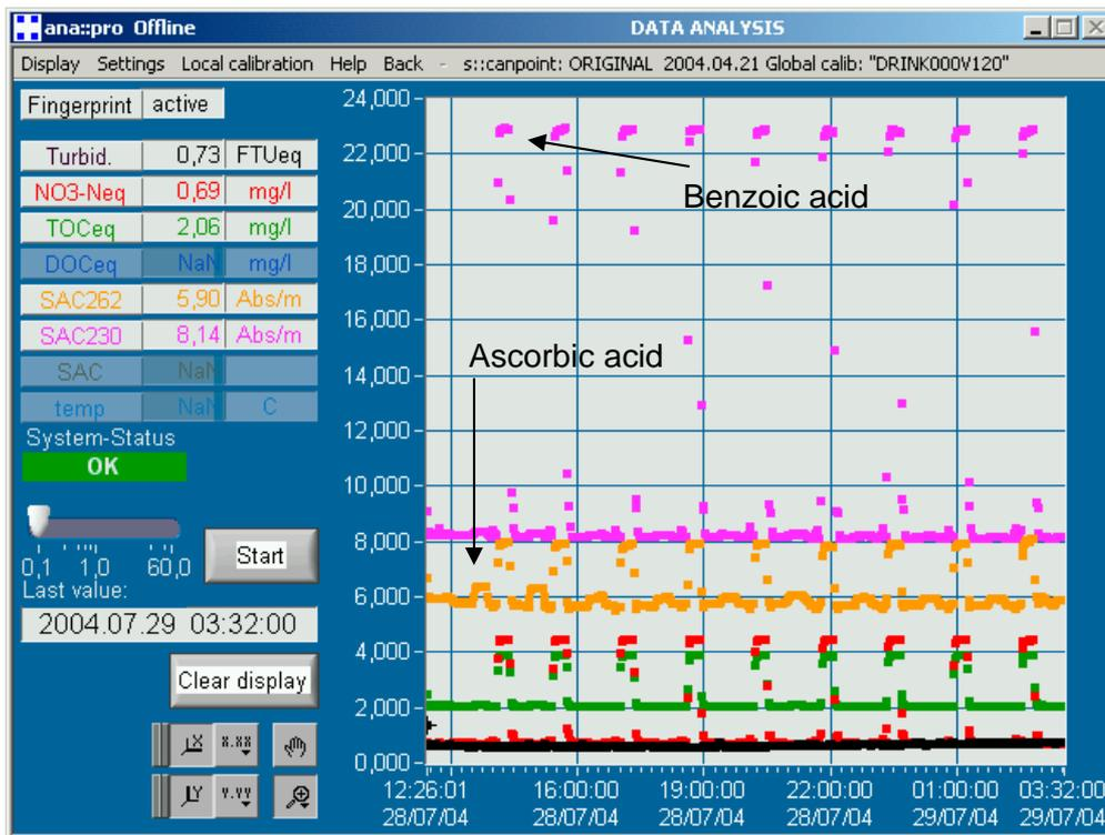
**Figure 3.7:** Monitoring drinking water with alternating additions of ascorbic and (0.2 mg/L) benzoic acid (5 mg/L).
