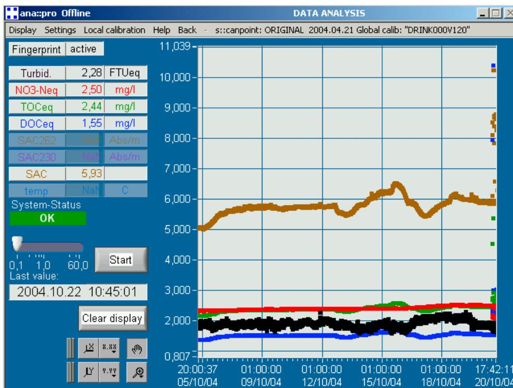
**Figure 3.12:** Scale of the natural variations in the pre-treated water in comparison with the spiking of ascorbic acid at 2 mg/L (far right).
