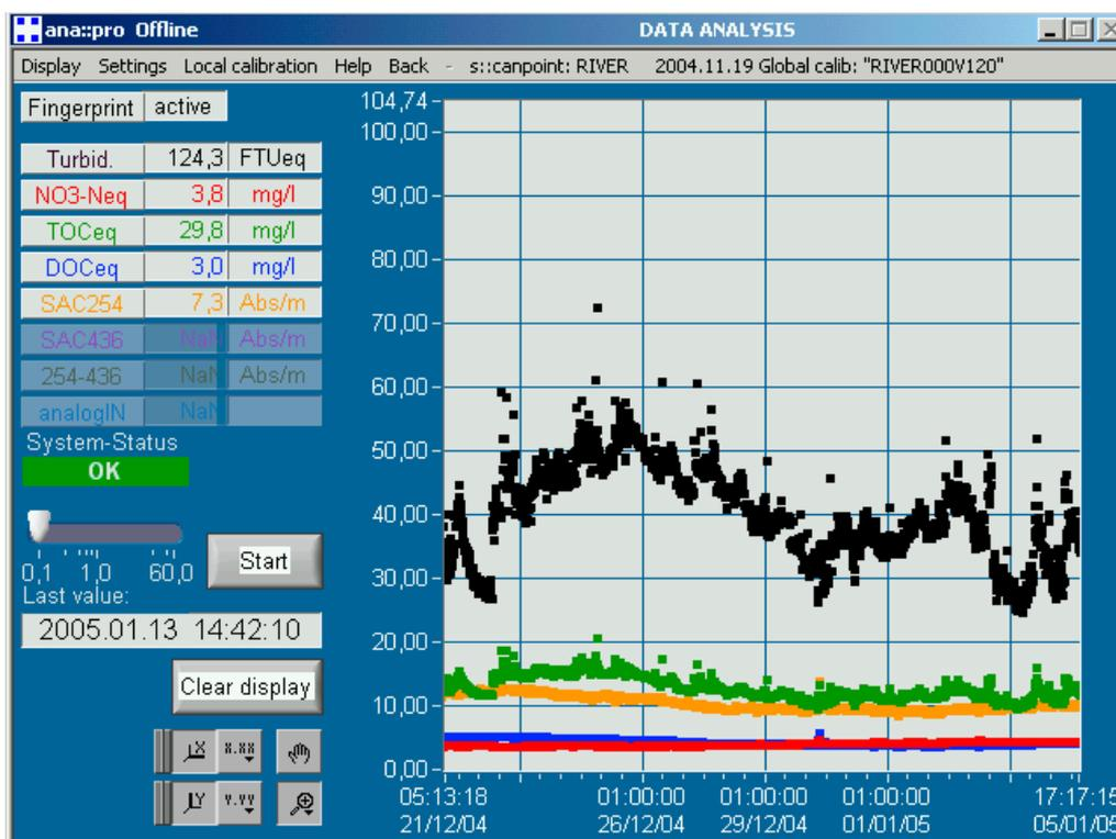
Figure 3.10: Strong fluctuations in turbidity observed when monitoring surface water
