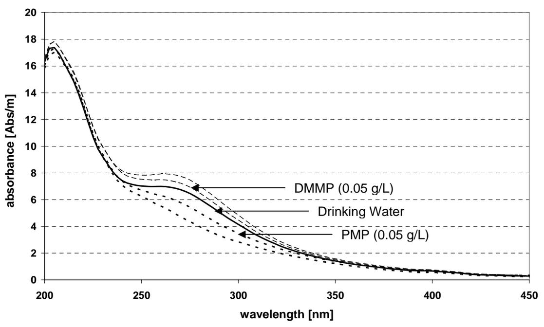
Figure 3.6: Detection of nerve gas simulants in drinking water. Fingerprints of water contaminated with simulants are shown for 0.05 and 0.1 g/L.
