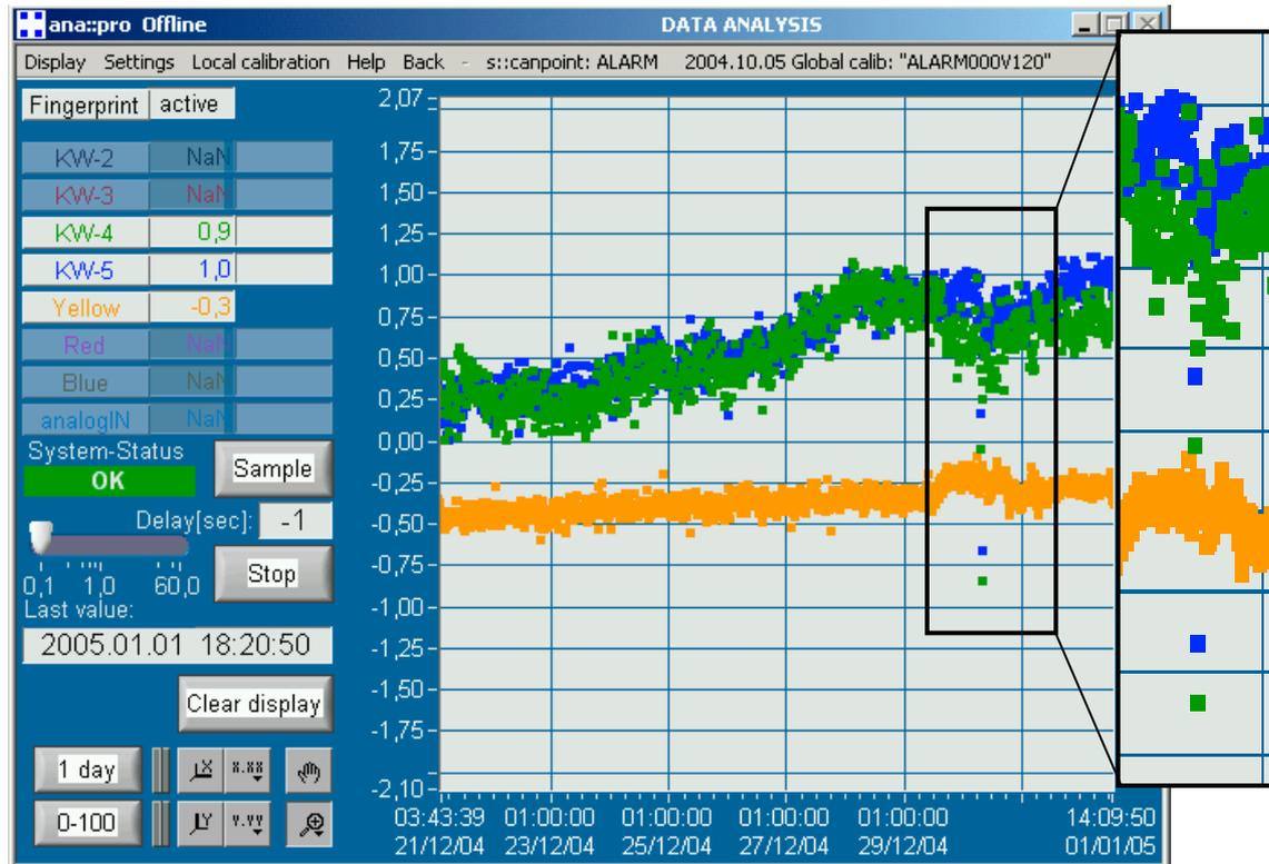
Figure 3.14: Response of alarm parameters to changing water quality.
