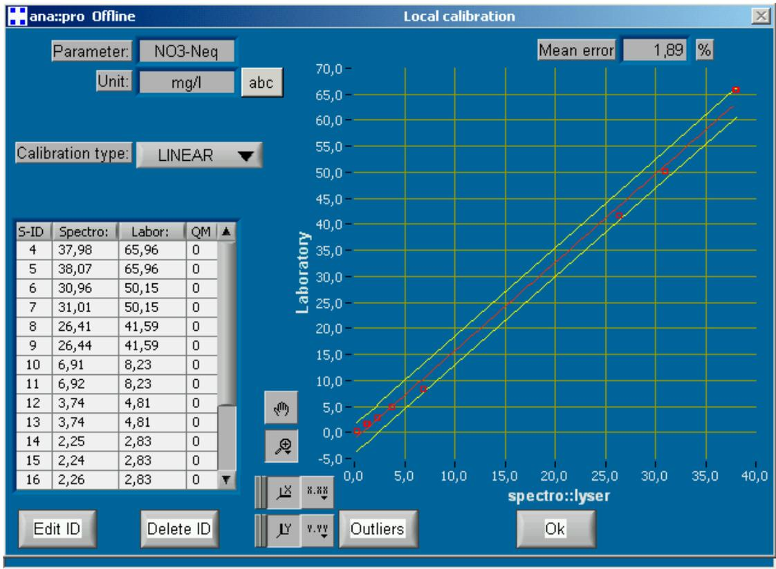
Figure 3.2: calibration curve obtained for nitrate in milliQ using a 10 mm path length.
