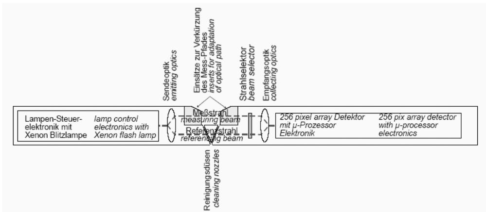
**Figure 2.2:** Schematic representation of the spectrophotometer.
