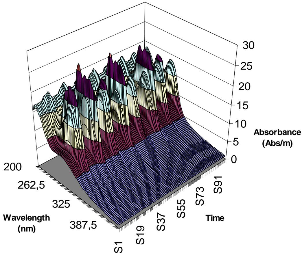
**Figure 3.13:** 3D-plot of the fingerprint spectra recorded over a period of 1 day during which benzoic acid and ascorbic acid were sub sequentially spiked every 6 hours.
