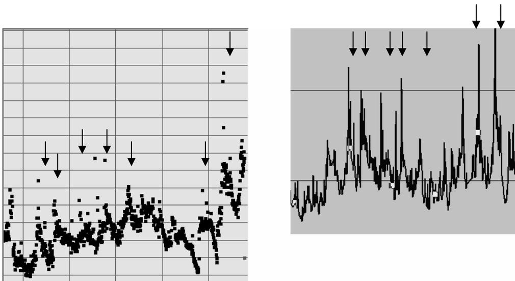
**Figure 3.11:** Comparison of measurement data, left: Spectro::lyser, right Hach turbidity meter.
