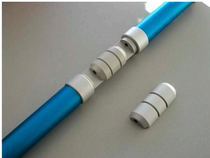
**Figure 3.1:** The 100 mm probe equipped with a 65 mm insert. A 90 mm is pictured besides the probe.
