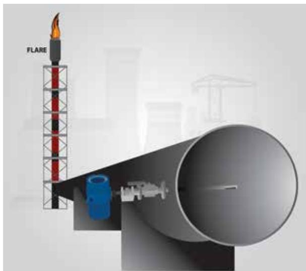
**Figure 3.** Kurz flow meter for flare applications.
