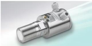
These detectors are no barrier for the bulk materials, they are in level of the duct wall and replace "fork" type of movement detectors. These are often quickly eroded by moving bulk products.
