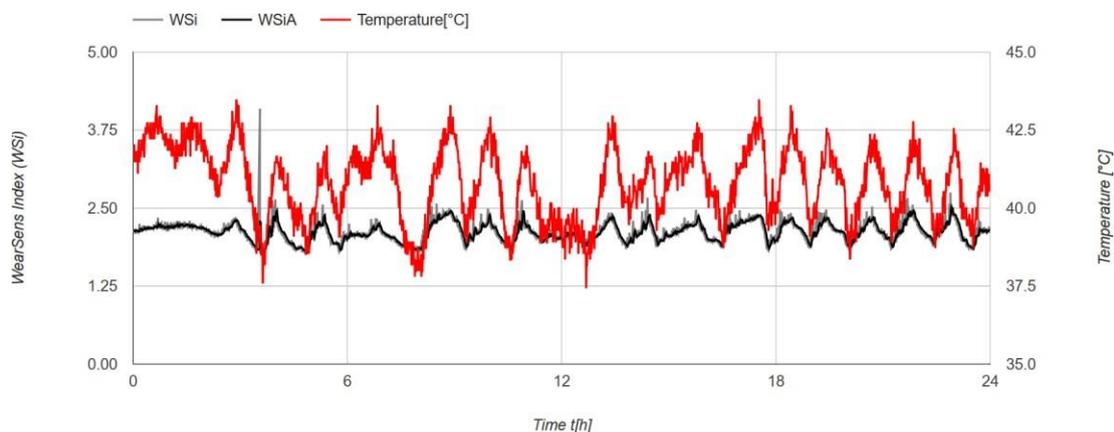
**Figure 7:** Time course of a measured WearSens® Index WS<sub>i</sub>, temperature T over 24 hours.
