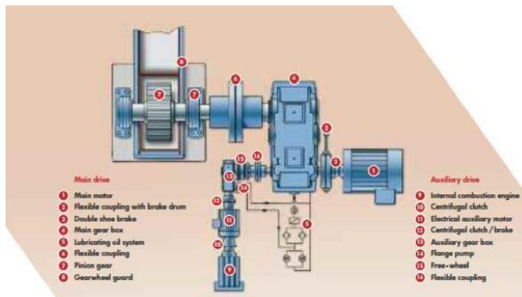
**Figure 1:** Typical Gear Drive Set Used in Cement Plants
