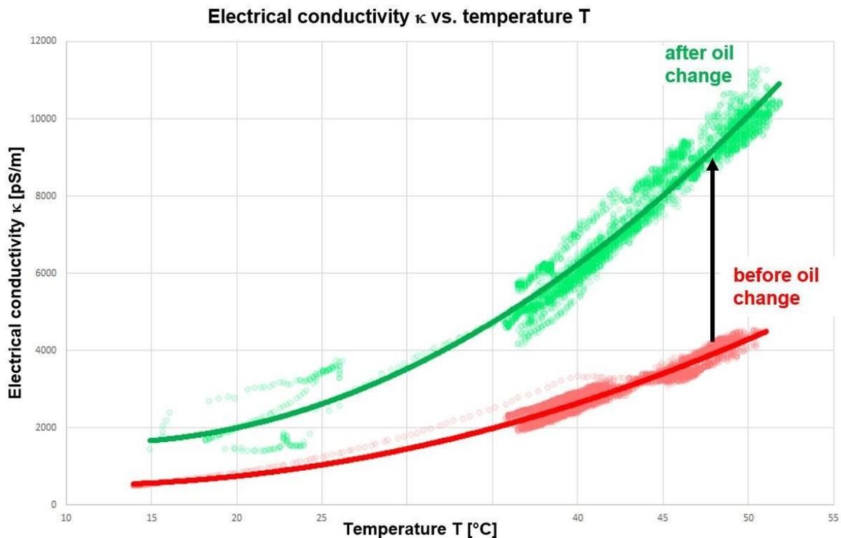
**Figure 8:** Temperature dependency of the electrical conductivity  $\kappa$  before (red) and after (green) the oil change.
