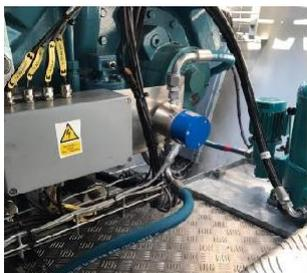
In the test and development phase of the gears and bearings on test benches, the sensor supplies essential statements on wear mechanisms. Correlation of test protocols results in component optimization.
