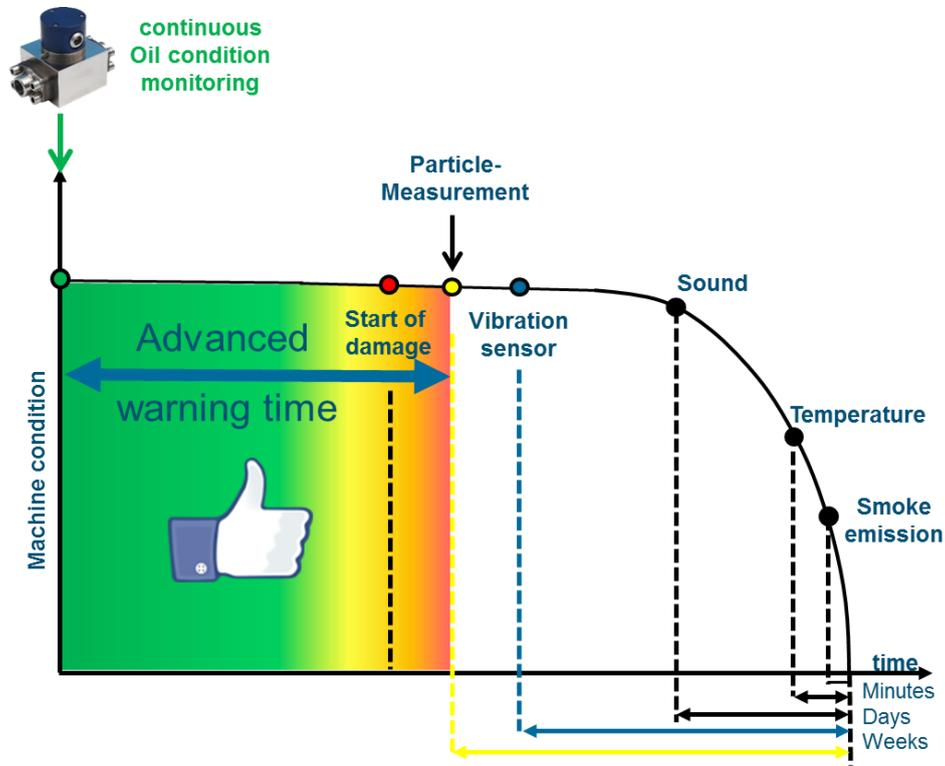
**Figure 4:** Existing sensor technologies such as optical particle measurement or vibration sensors can detect particles only **after** the occurrence of damage.
