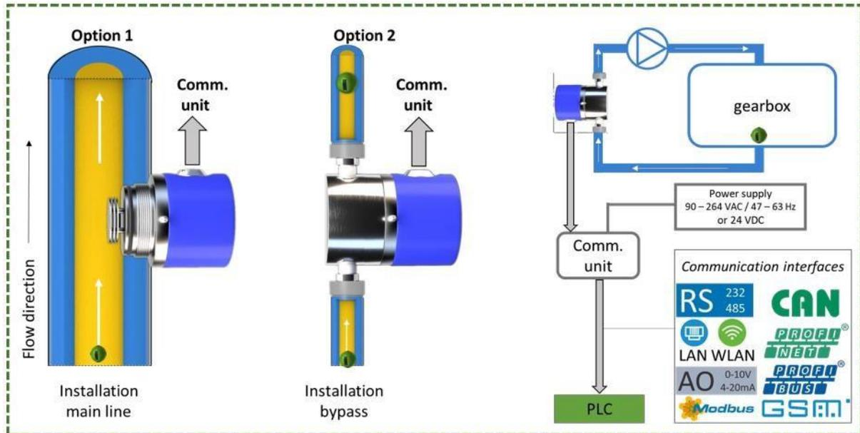
**Figure 5:** Installation scheme of the WearSens® WS 3000 sensor system.
