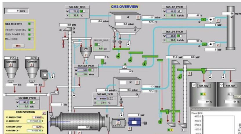
**Figure 3:** Process Visualization of a Typical Cement Plant
